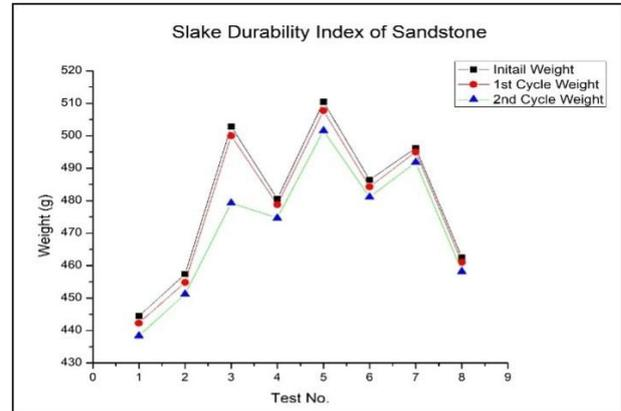
Figure 7. Sandstone Slake Durability Index
