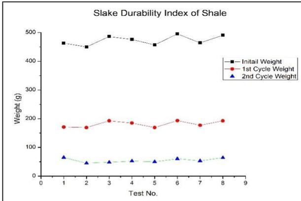
Figure 9. Shale Slake Durability Index
