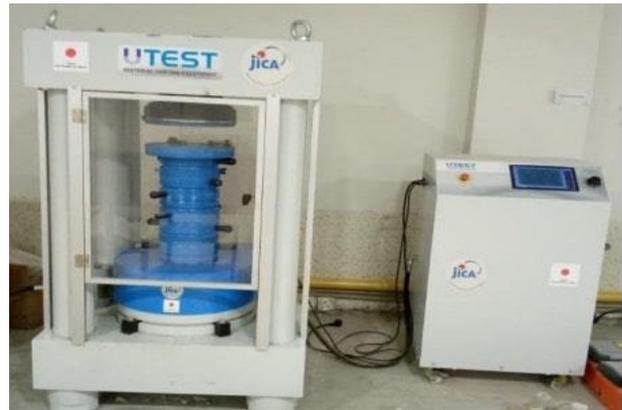
**Figure 5.** Uniaxial compressive (UCS) test Apparatus
