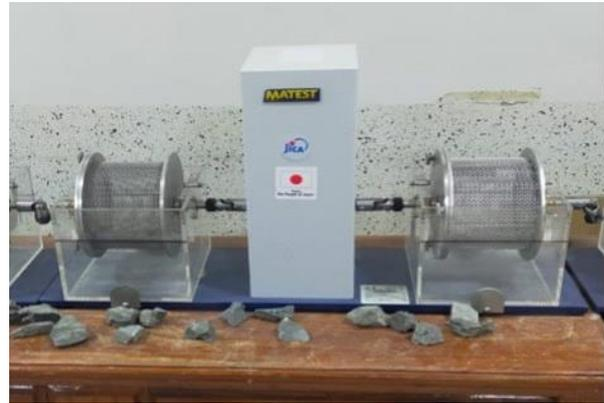
**Figure 4.** Slake durability index test Apparatus
