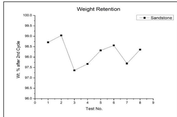
Figure 8. Sandstone Slake Durability Index
