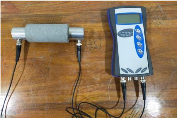
Figure 6. Ultrasonic pulse velocity (UPV) tester.
