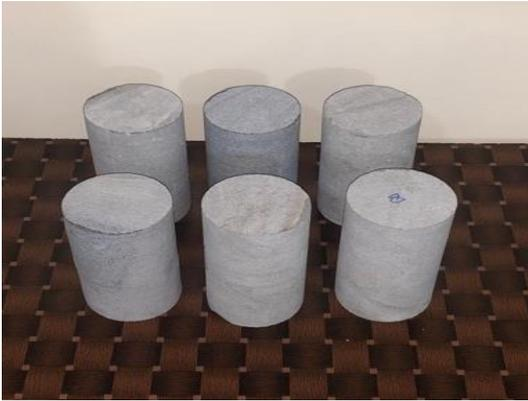
**Figure 3.** UCS testing core samples
