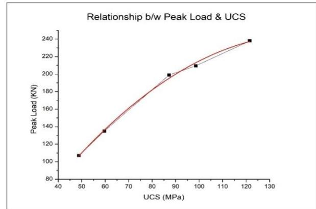
Figure 11. Relationship between Peak Load & Uniaxial Compressive Strength (UCS)
