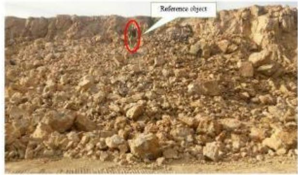
Figure 3: Blasted muck file of blast 2
