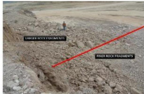
Figure 7: Blasted muck file of blast 3
