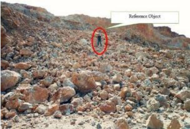
Figure 1: Blasted muck file of blast 1
