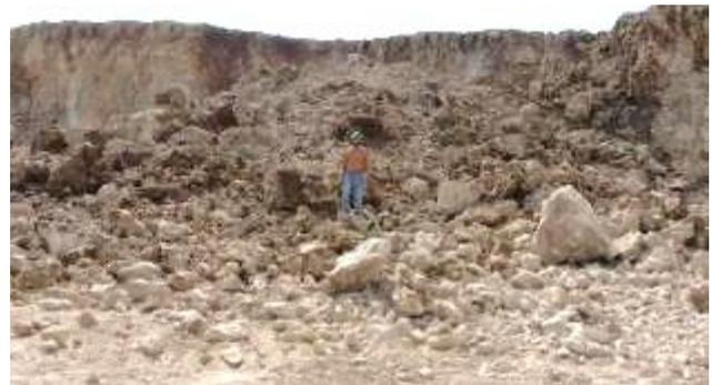
Figure 10: Blasted muck file of blast 4
