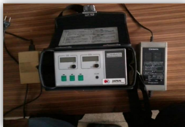
Figure 3. SIBATA CO 2 meter
